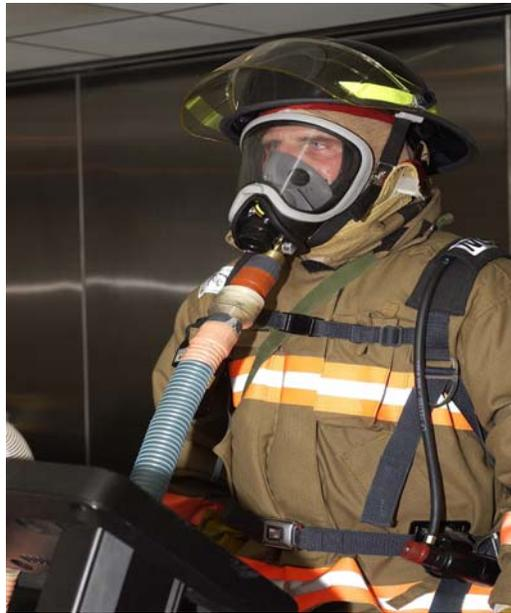
*Figure 5. Modified SCBA facepiece outtake valve with hose adaptor*
